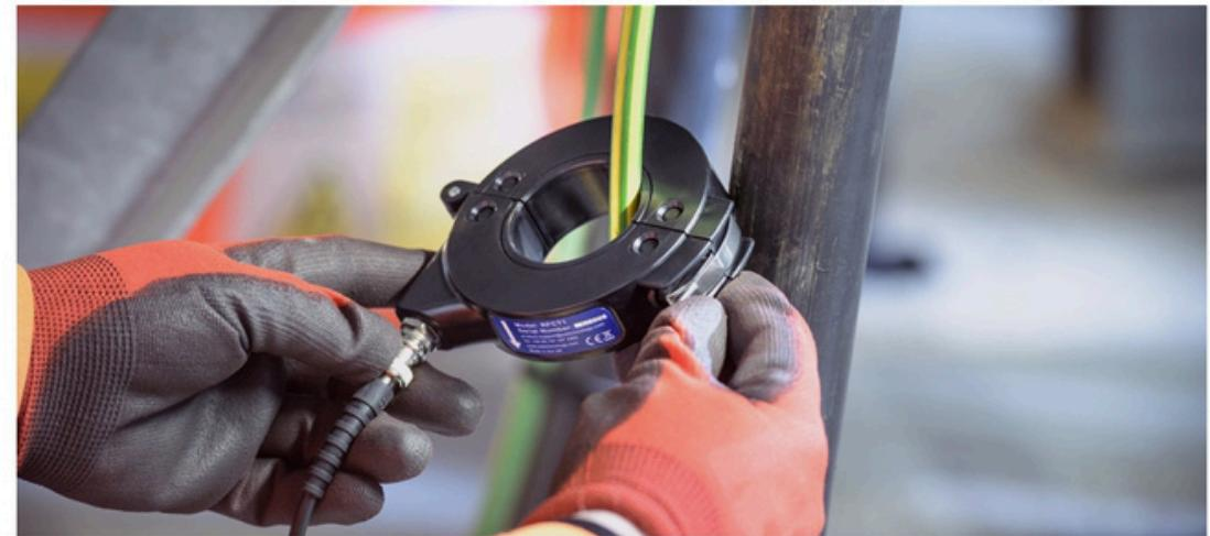
The **CableData Monitor®** allows us to continuously monitor and report to you on PD activity in live cable networks. This helps to reduce the need for disruptive maintenance shutdowns by highlighting high risk areas in ample time for repairs and replacements to be made if necessary. The system is a fully integrated modular system with up to 20 nodes and each system is capable of monitoring up to 180 cables.
